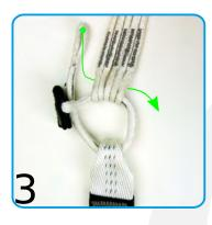
Pass the BLINK through the suspension lines loop a second time
