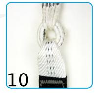
Pull suspension lines and the riser apart, strongly, to setup the BLINK
